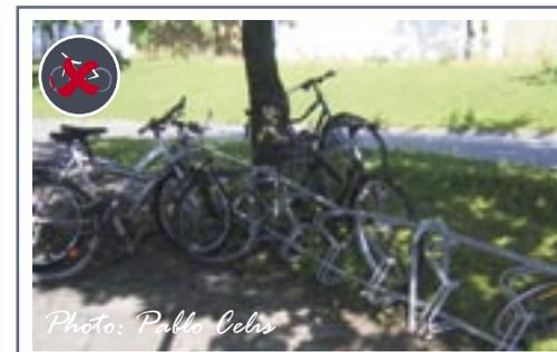
Non-wedge-shaped butterfly rack – only suitable for wide tyres, and ordinary bicycles fall over easily.
