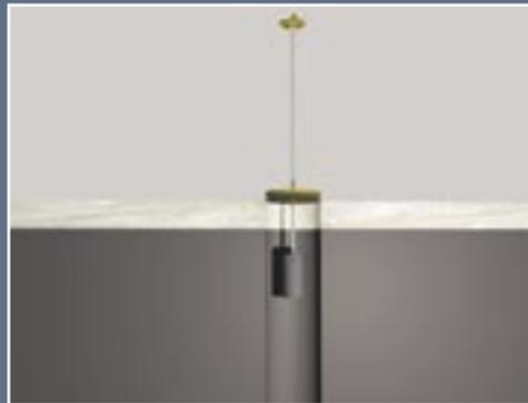
*When the bicycle key is used, the weight adjusts the length of the wire and maintains tension.*
